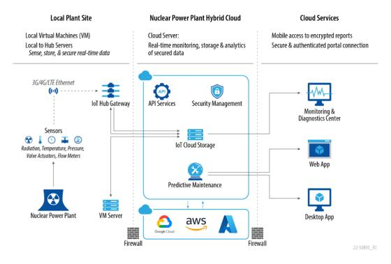
Figure 1. Proposed high-level architecture of the hybrid cloud.
