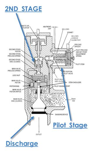
Figure 2. SRV diagram marking the sensor placements [11].
