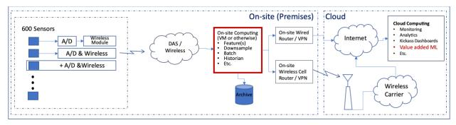
Figure 6. Example of a DAS network.
