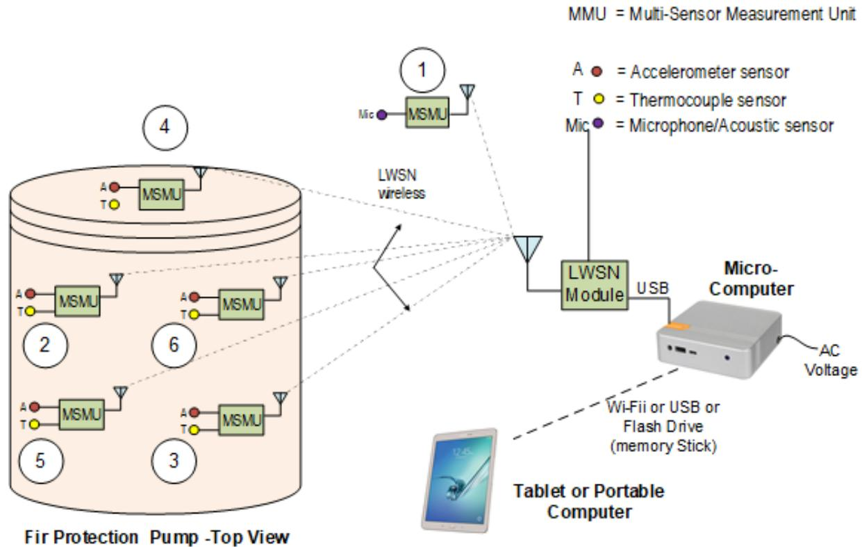
Figure 3. Implemented layout of the MSMU setup.
