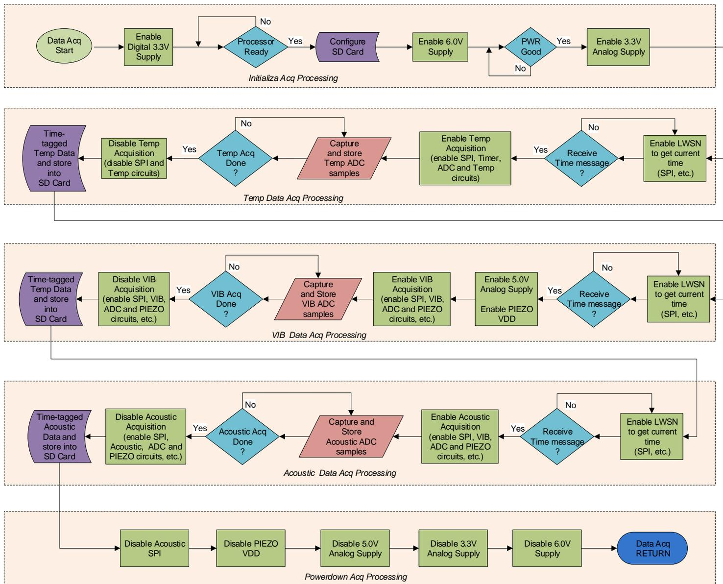
Figure 9. Data-acquisition process flow chart.
