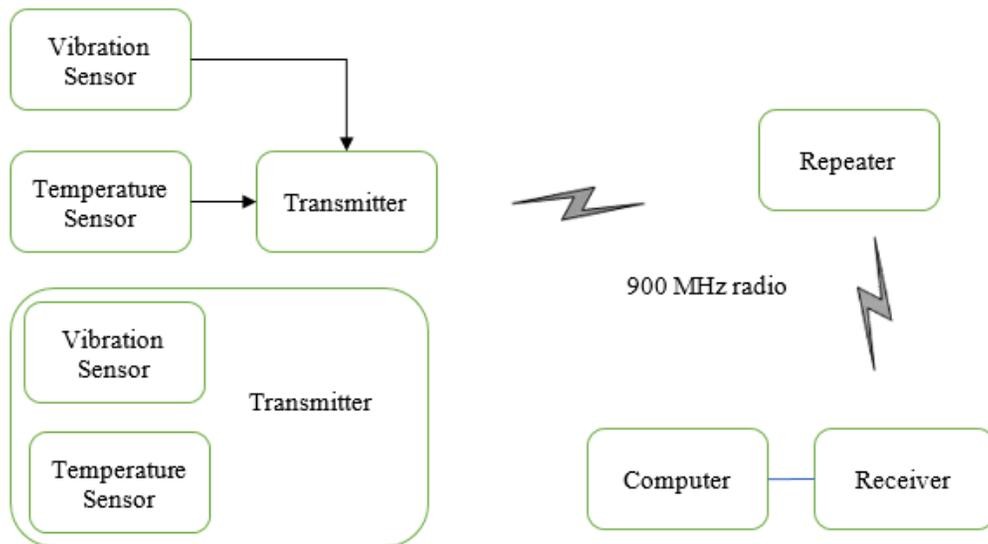
Figure 18. Continuous monitoring multi-sensor system layout.
