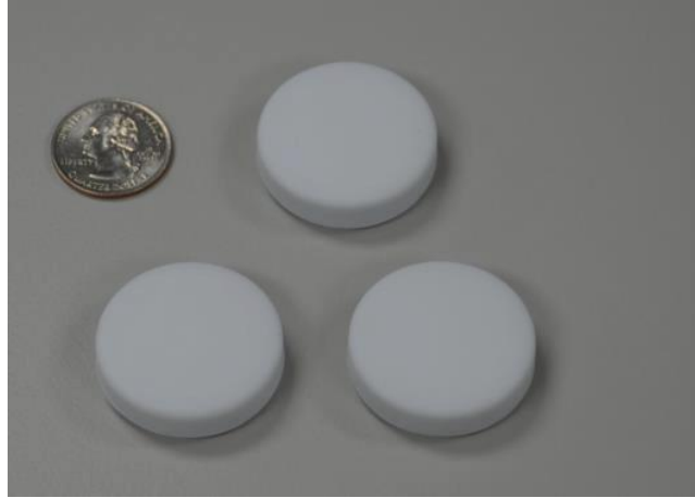
Figure 2. Bluetooth-enabled microcontrollers used as beacons (Al Rashdan et al. 2017).
