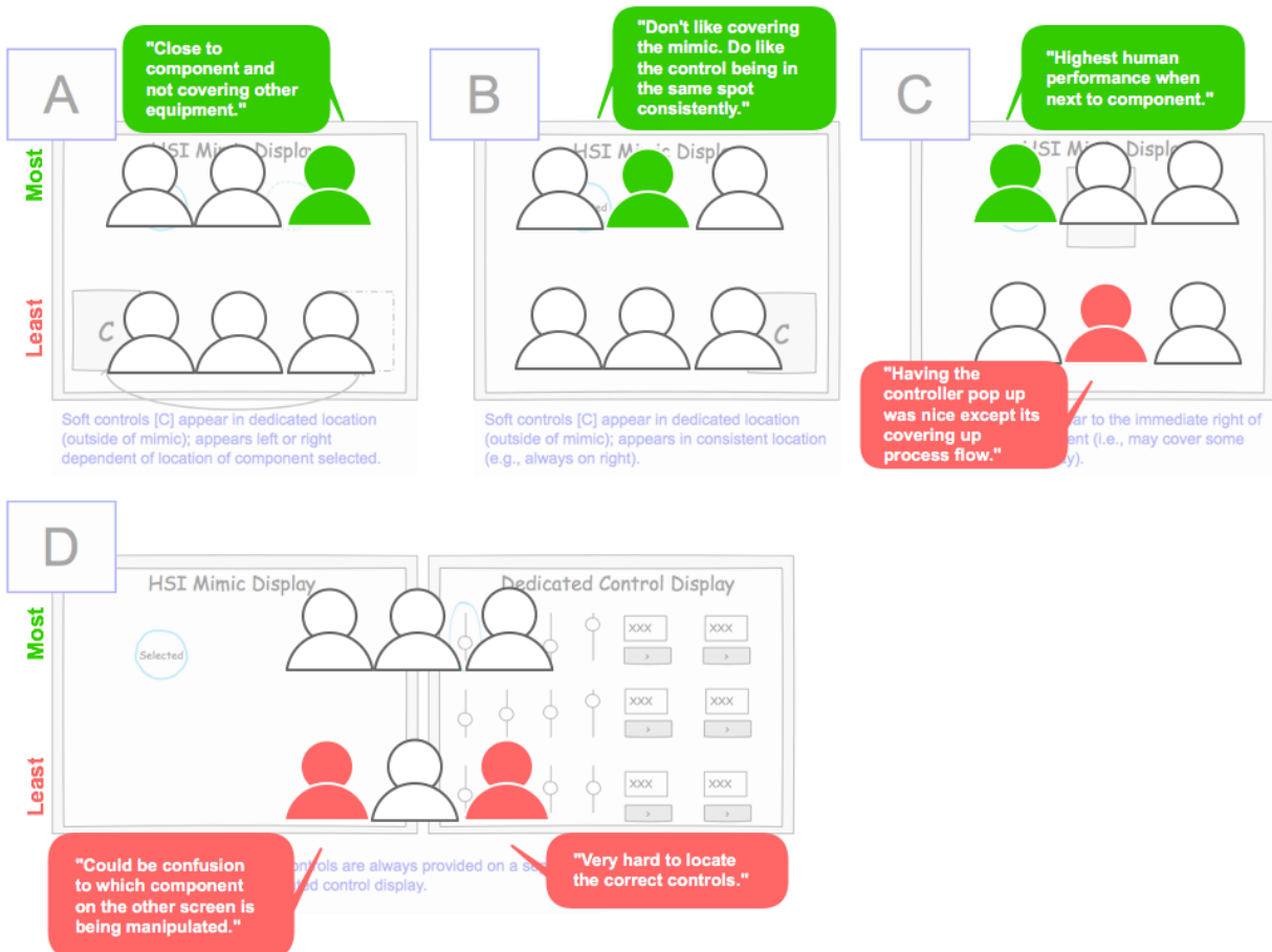
Figure 52. Most and least preferred soft control design schemes from main control room operators.
