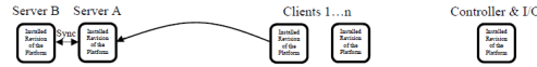
Figure 15. Step 1: Synchronization of Configurations Between Servers is Performed and All Clients are Connected to Server A.
