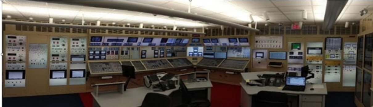
Figure 5. Leveraging glasstop simulator for I&C design and procedure development in addition to operator training.
