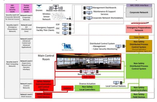
Figure 6. Simplified digital infrastructure (adapted from INL/EXT-21-64580).
