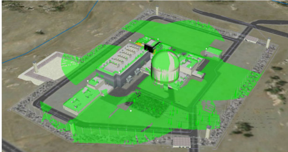
Notional Dante ViewShed Visualization Showing Double Firepower Coverage Areas on the Fictional Lone Pine Nuclear Power Plant Site for Modeling External ROWS Placements
