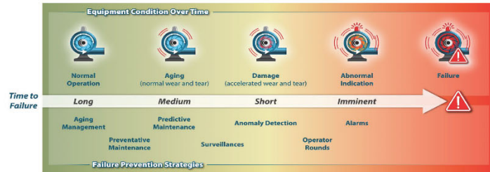
Role of anomaly detection in prevention of failure escalation
