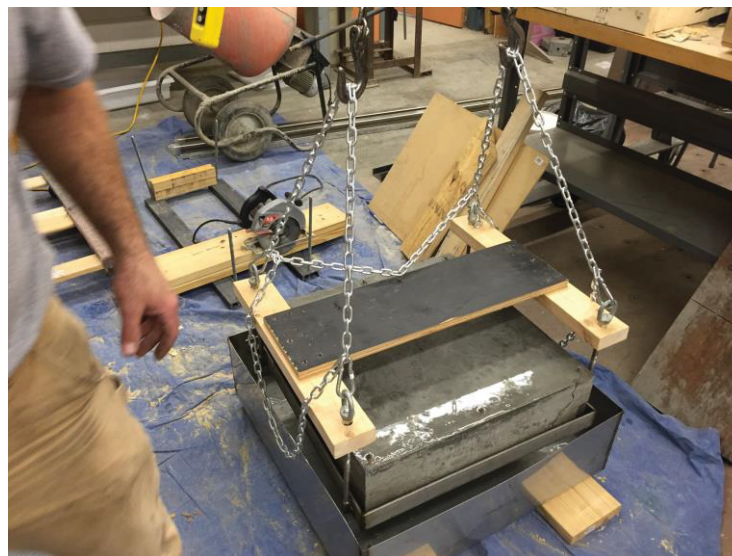
Figure 5. Slab sitting on the frame and being lowered into the tub.
