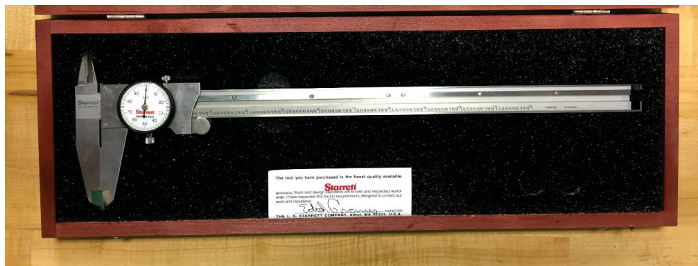
Figure 10. Calipers used for mechanical deformation measurements.
