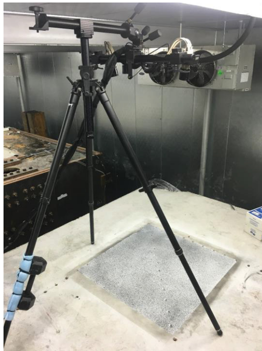
Figure 56. DIC camera support installation over the area of interest.
