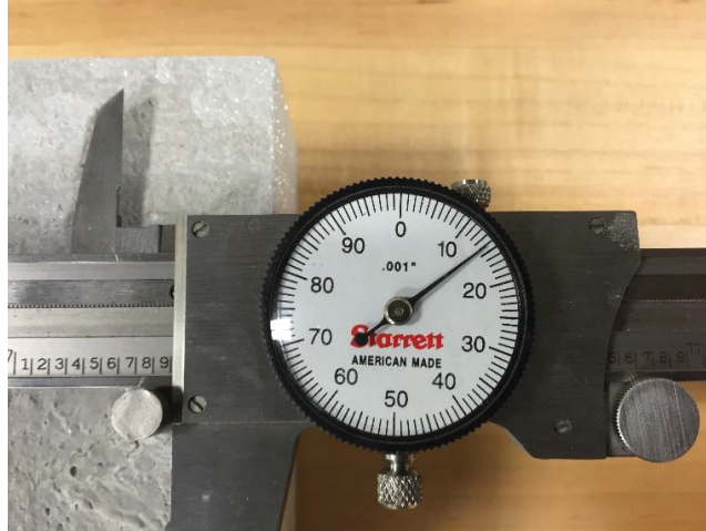
Figure 11. Calipers being used to measure the distance between nails.
