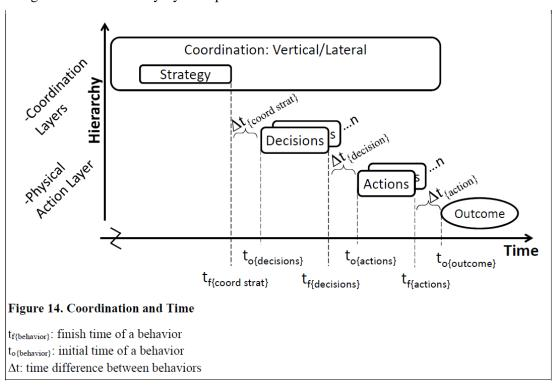
Figure 12. Modified SCS (from Johnson, 2017, Figure 14; Used by permission of author).
