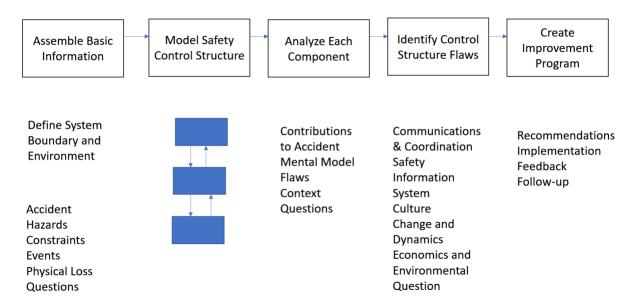
Figure 9. Major components of CAST analysis (Modified from Leveson, 2019, p. 34).
