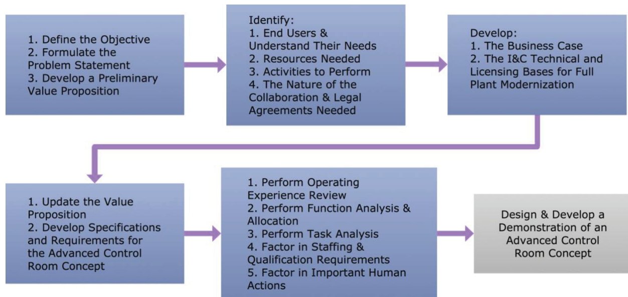
Figure 8. Proposed Planning & Analysis Activities Needed to Design & Develop an Advanced Control Room Concept
