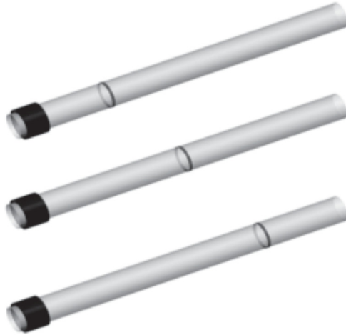
Figure 7. Axisymmetric GW inspection displaying wave propagation at specific times along the length of a pipe [29].
