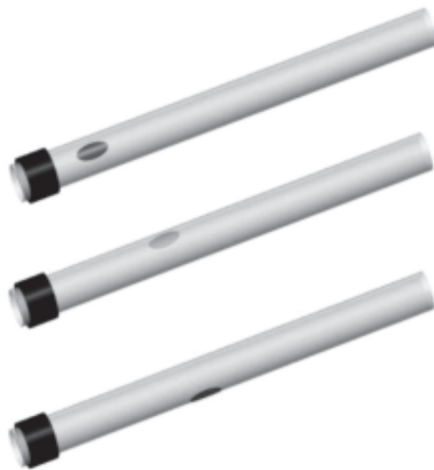
Figure 8. Focused GW inspection displaying focused beam at specific times as it moves around and along the length of pipe [29].
