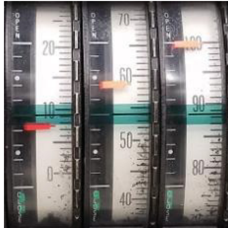
Figure 19. Example of current control room “green band function” cited by one operator’s feedback.
