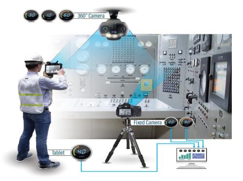
Figure 1. Automated gauge reading enables any camera to be used to log several gauges autonomously.
