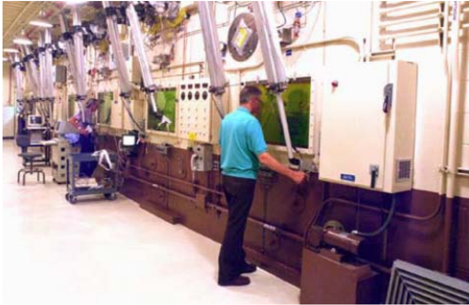
Figure 33. HFEF Hot Cell Windows and Manipulators
