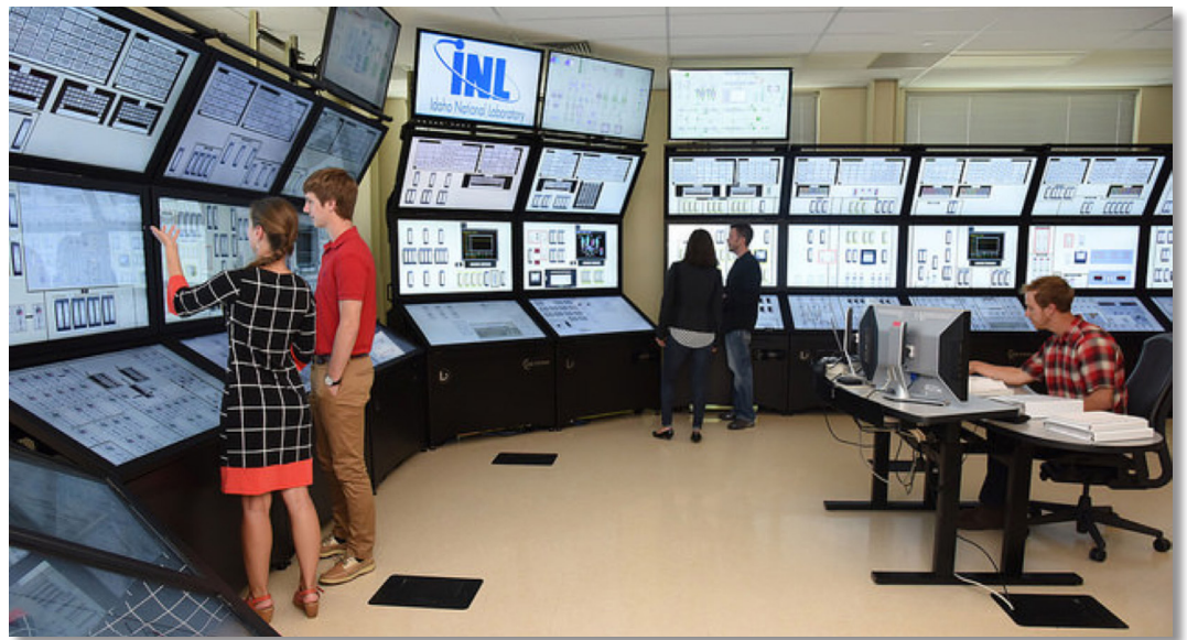
Human factors researchers collect data in the HSSL full-scale and full-scope simulation facility.
