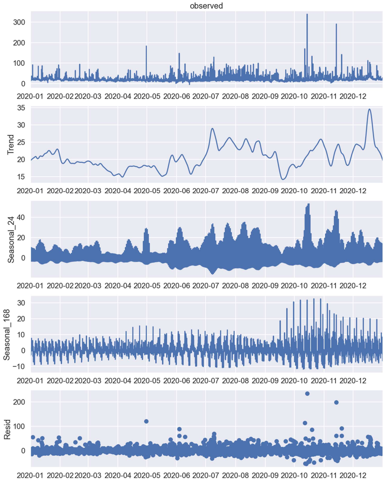
Figure 28. The decomposition of hourly RT-LMP at Braidwood NPP in 2020 using MSTL. Each panel represents the original data, the trend, the daily seasonality, the weekly seasonality, and the remainder respectively.
