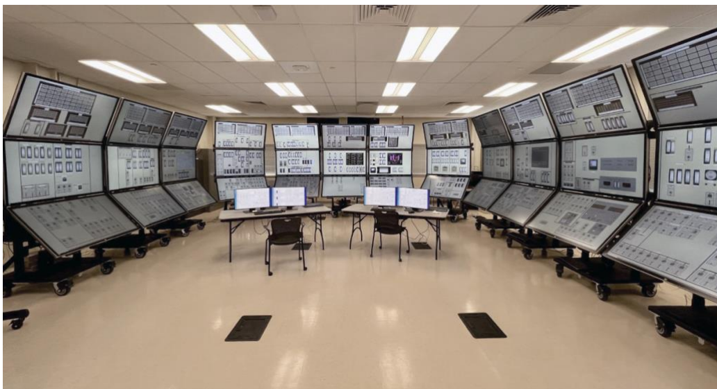
Figure 1. The INL HSSL showing the GSE GPWR simulator analog control room panels represented virtually on touch screen displays.
