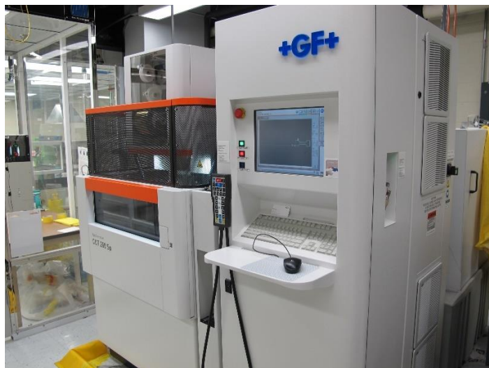
Figure 6. EDM system installed in LAMDA to manufacture specimens from radioactive material.
