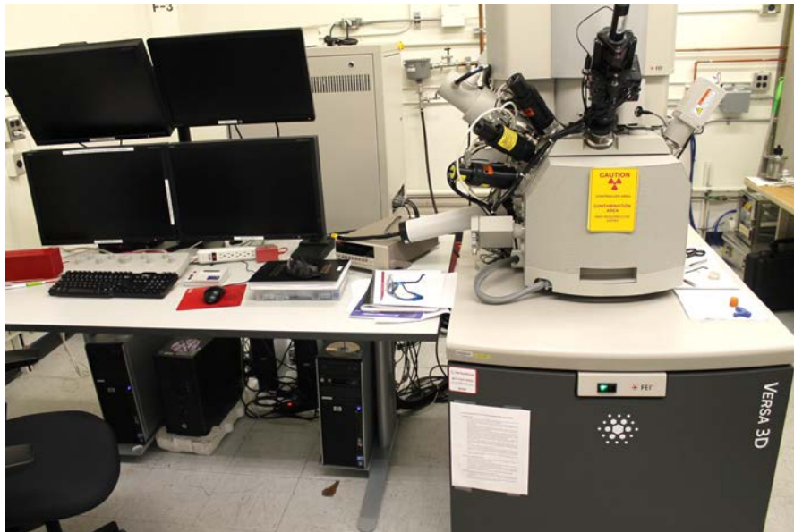
Figure 1. General view of the VERSA 3D dual beam (scanning electron microscope and ion beam).
