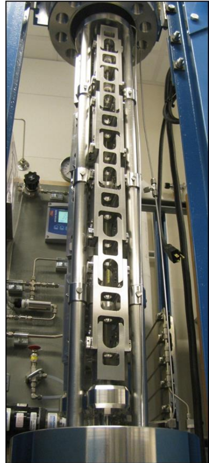
Figure 2. Crack initiation test system load train at PNNL in the (a) small SCC initiation test system with capacity of testing up to 6 fully instrumented specimens and the (b) large SCC initiation test system with capacity of testing up to 24 instrumented specimens and up to 36 specimens in total.
