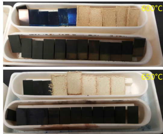
Figure 2. Photos of the tested alloy coupons in crucibles exposed to steam at 600 and 650°C for 500 h.
