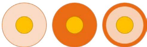
Figure 12. Schematic insulated conductor cross-sections illustrating unaged cable (Left), homogeneously aged cable (no DLO) (Center), and heterogeneously aged cable exhibiting DLO (Right).
