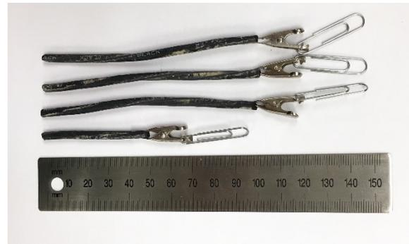
Figure 4. BIW EPR/CSPE (BE15) specimen set
