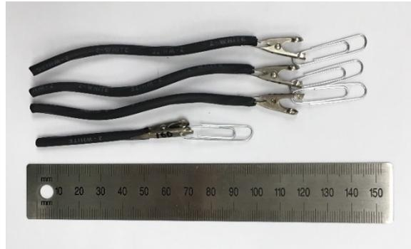
Figure 6. Okonite EPR (OE34) specimen set
