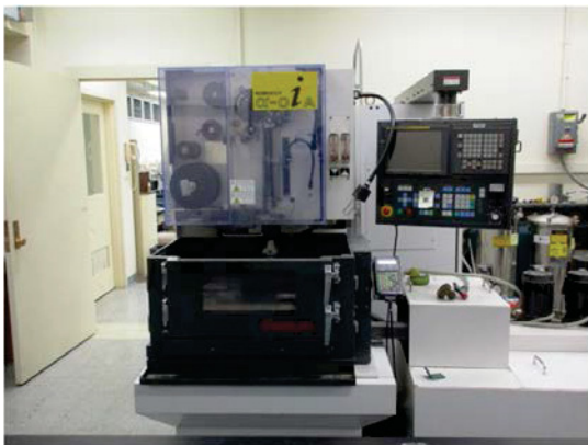
Figure 4: Wire EDM machine (L), Wire EDM close-up (R)
