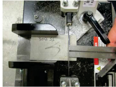
Figure 7: Band saw for coupon cut (L), Coupon setup with the band saw (R)
