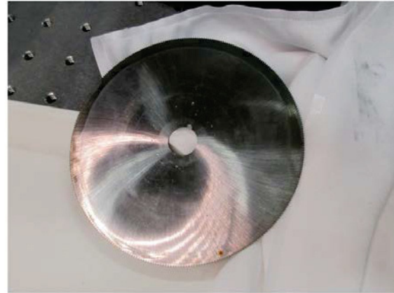
Figure 3: Slow saw test cut setup (L), Worn jeweler's slotting saw blade (R)
