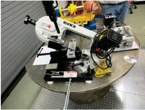
Figure 7: Band saw for coupon cut (L), Coupon setup with the band saw (R)
