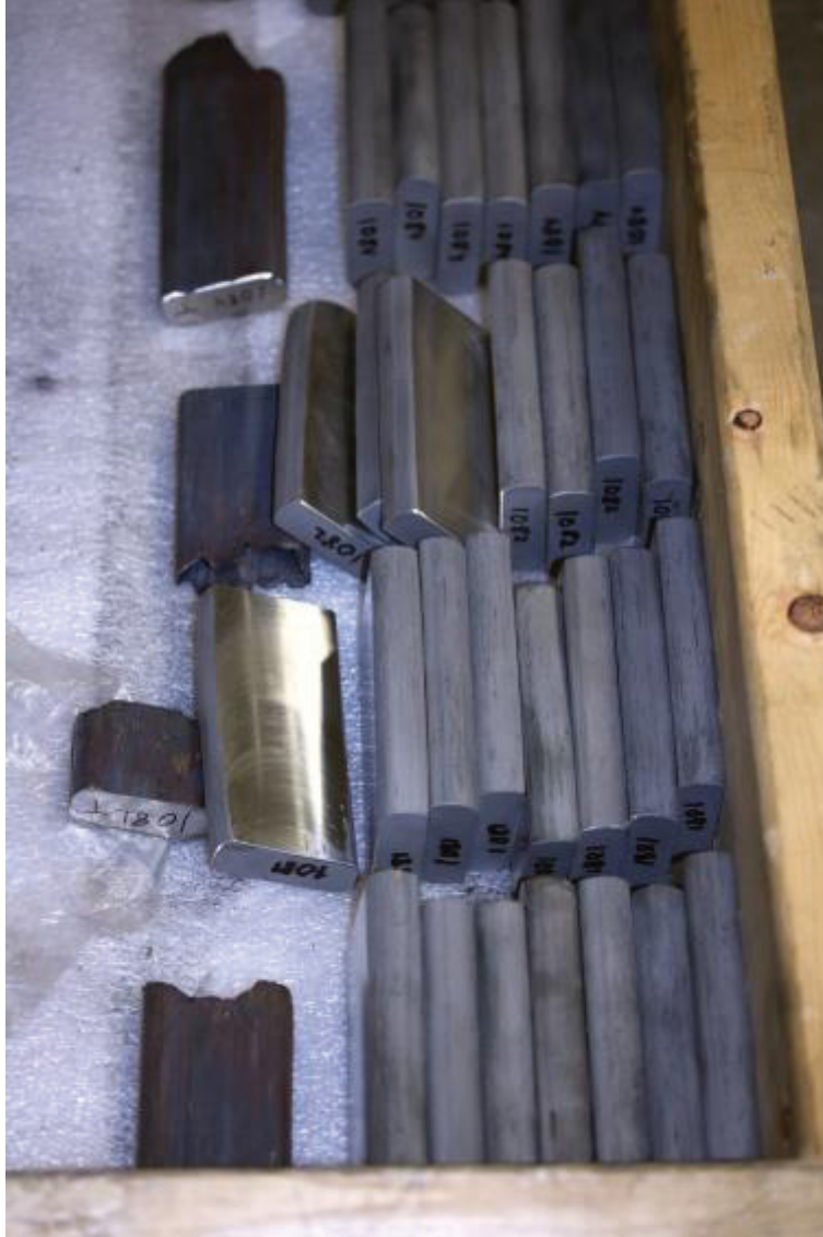
Figure 15. Extruded and cut billets ready for hot rolling
