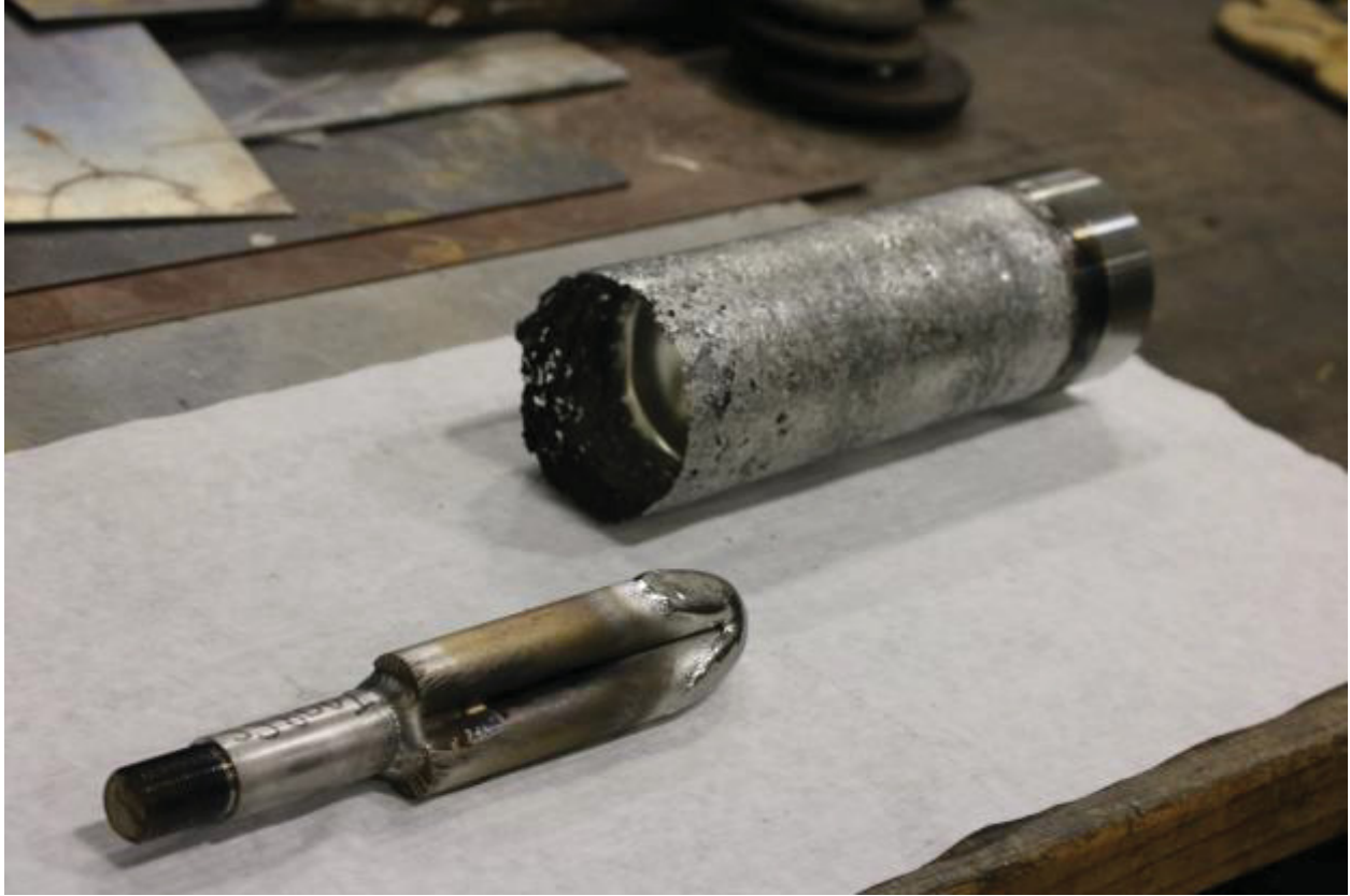
Figure 14. Completed VAR casting and remaining electrode stub
