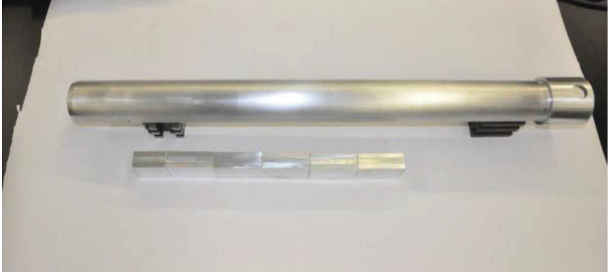
Figure 4. Photo of specimen holder, irradiation specimens and height spacer prior to final assembly
