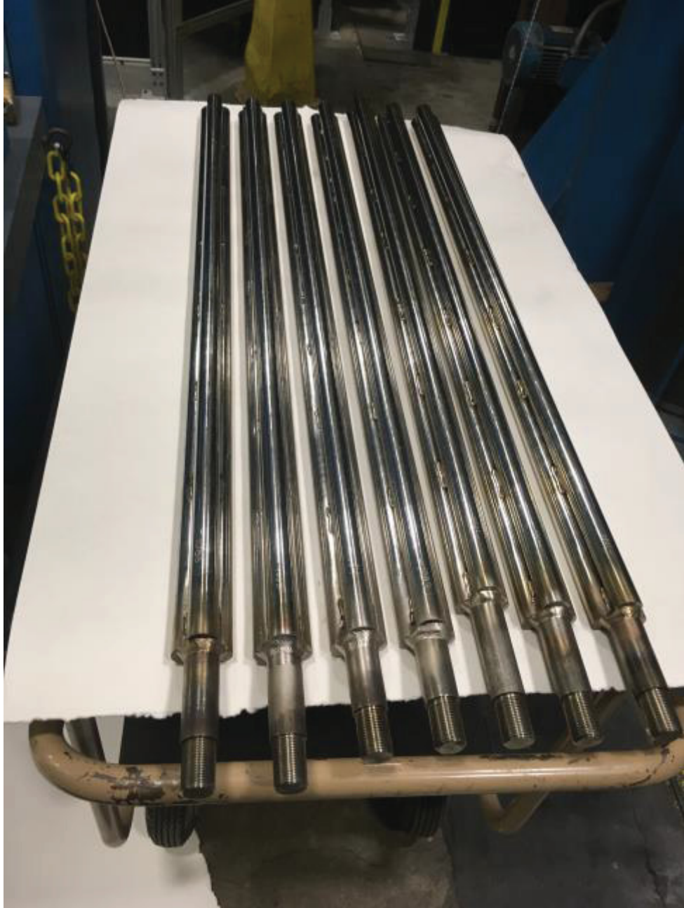
Figure 13. Electrode Assemblies of 304L and 316L with controlled boron additions prior to VAR processing
