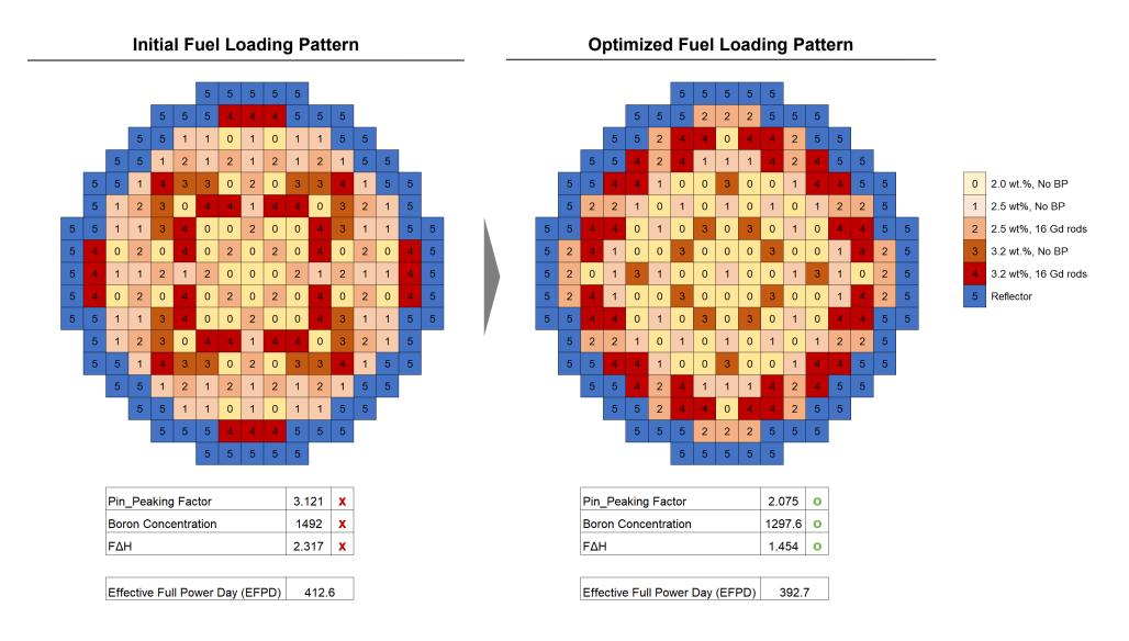
A generic PWR reactor core is used for the demonstration
