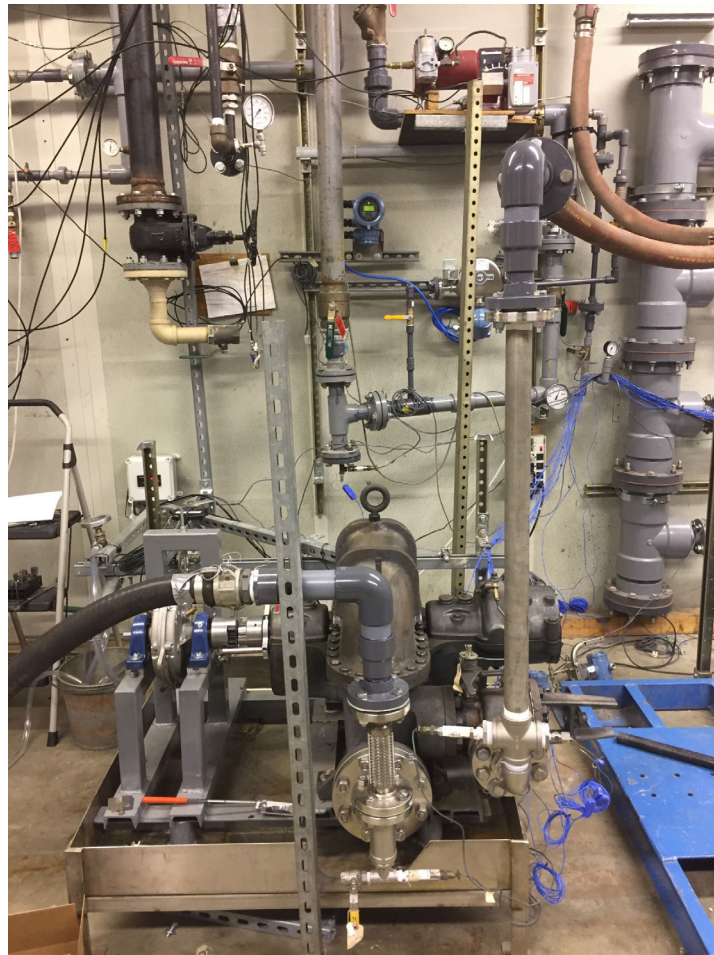
Figure 1. Experimental Setup for Air and Air-Water Tests of Terry ZS-1 Turbine.
