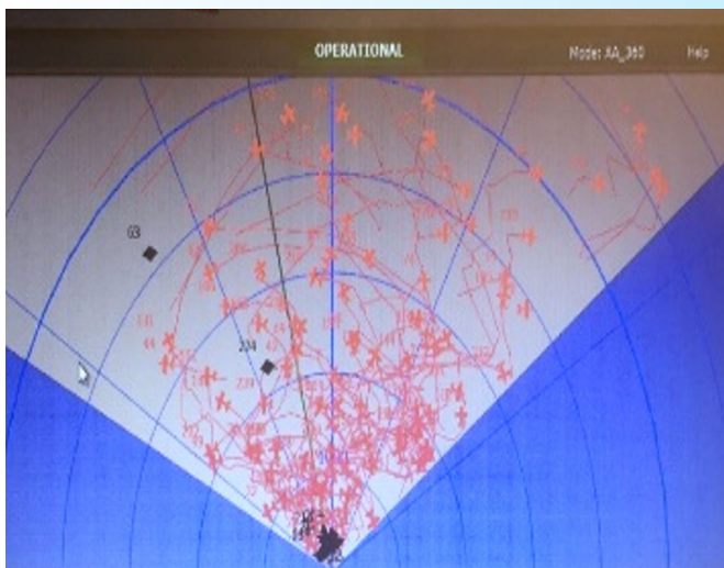
Figure 1. Nuisance alarms generated during a light rain shower.
