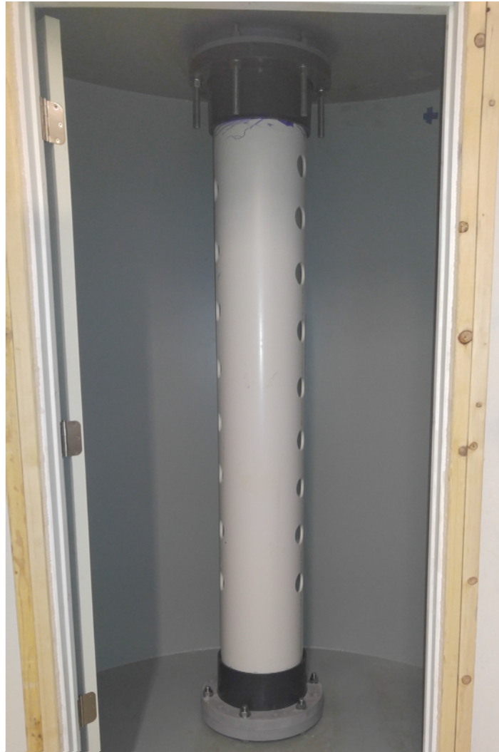
Figure 9. PET stand pipe for 12-in line.
