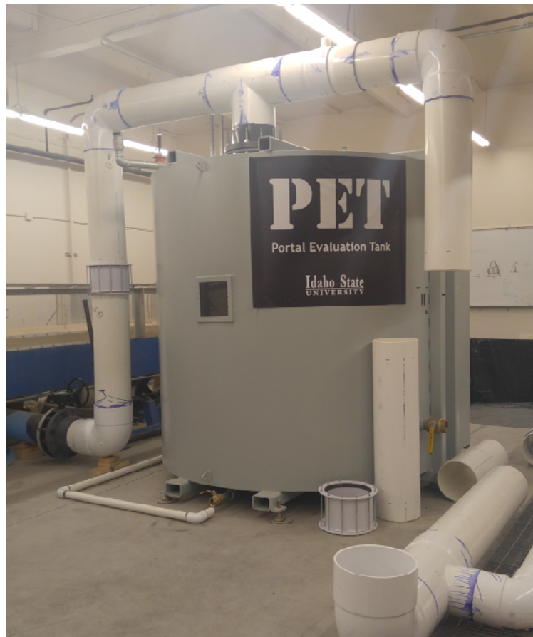
Figure 7. PET high flow piping.
