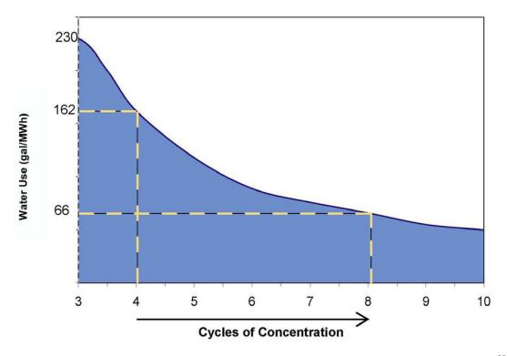
Figure 2-2: Typical Water Losses from Cooling Towers, at Varying Cycles of Concentration, EPRI<sup>25</sup>
