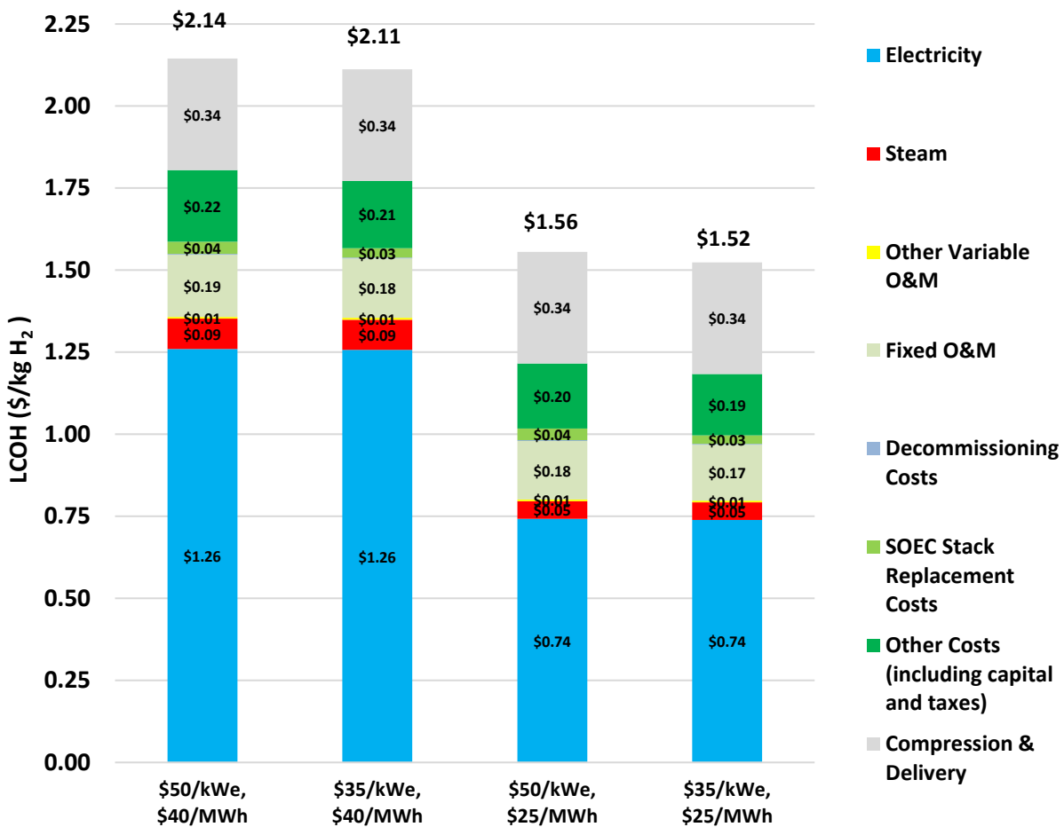
Figure 17. H 2 production cost contribution for four HTE cases (534-tpd H 2 production at 92.4 OCF without capacity payment).
