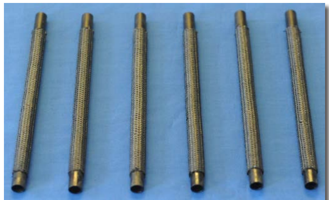
Prototype SiC ceramic matrix composite testing rods.
