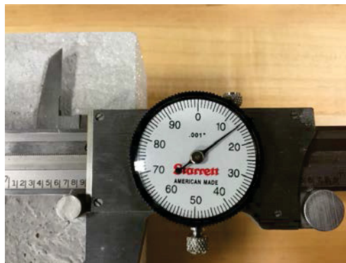
Figure 20. Measuring the distance between nails on a brick.
