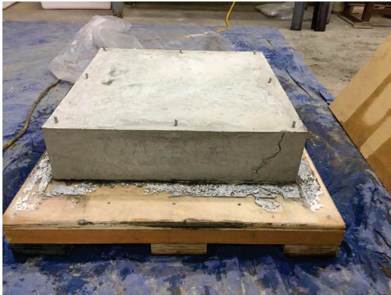
Figure 7. 2-ft \times 2-ft \times 6-in. cement slab.
