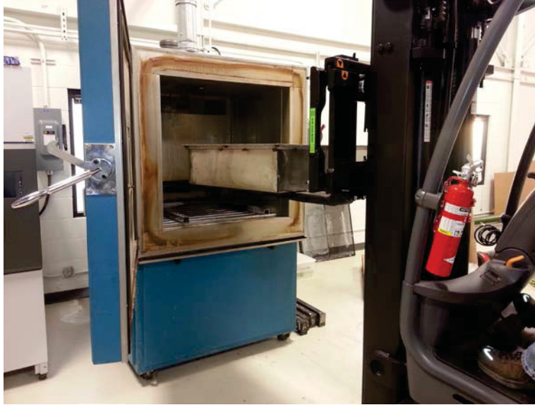
Figure 11. Slab being placed in the oven for accelerated curing.
