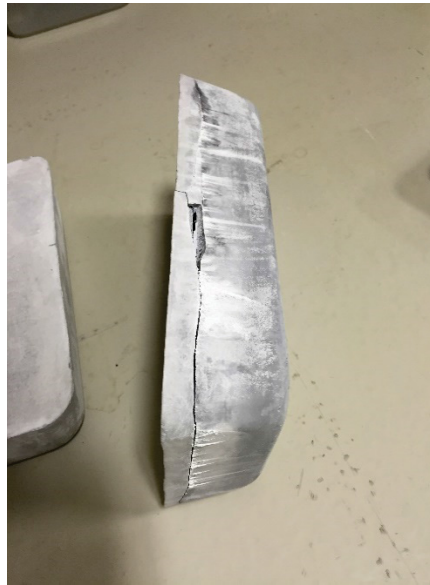
Figure 3. Brick B2 showing whitish effluent (ASR gel).
