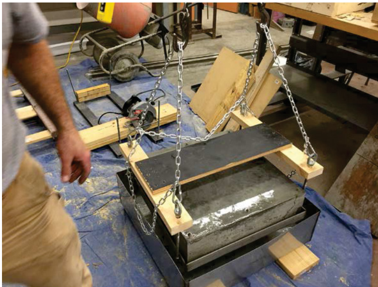
Figure 10. Slab sitting on the frame being lowered into the tub.
