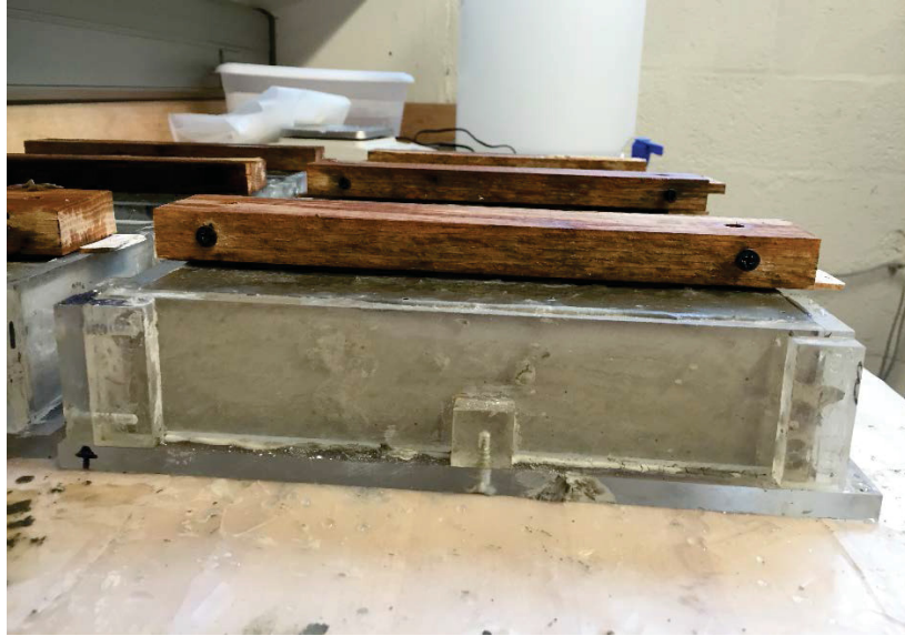
Figure 6. Stainless steel pegs being inserted during casting.
