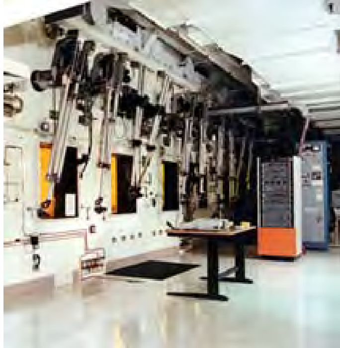
Figure 36. Work area in the ORNL Irradiated Materials Examination and Testing (IMET) facility facing the examination cells, showing manipulator controls for the remote handling of highly irradiated materials.
