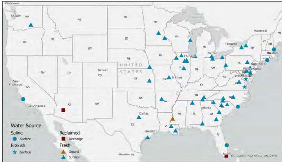
Figure 19. Commercial nuclear fleet cooling water source types. Data source: IEA.
