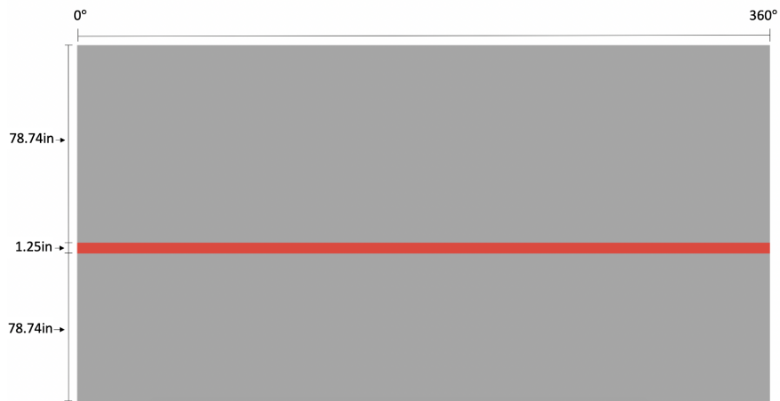
(c) Full beltline region of RPV consisting of forgings and weld
