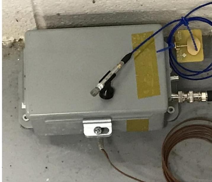
Figure 15. Acoustics MSMU installation in the fire protection room.
