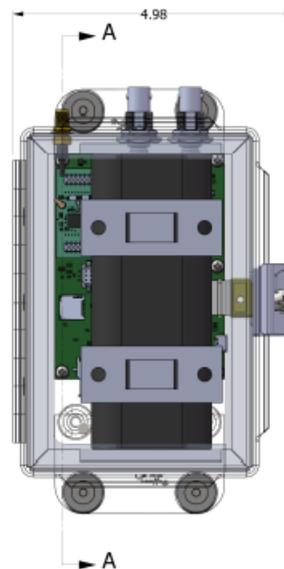
(b) Holder internal design showing the internal parts.
