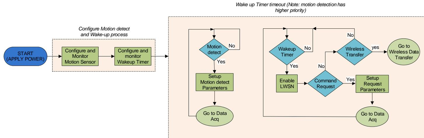
Figure 7. Monitoring motion and sleep-timer setup flow chart.
