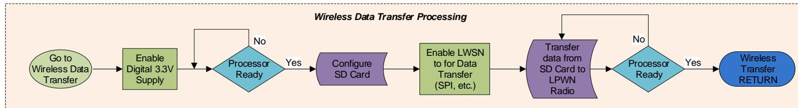
Figure 8. Wireless data-transfer flow chart.
