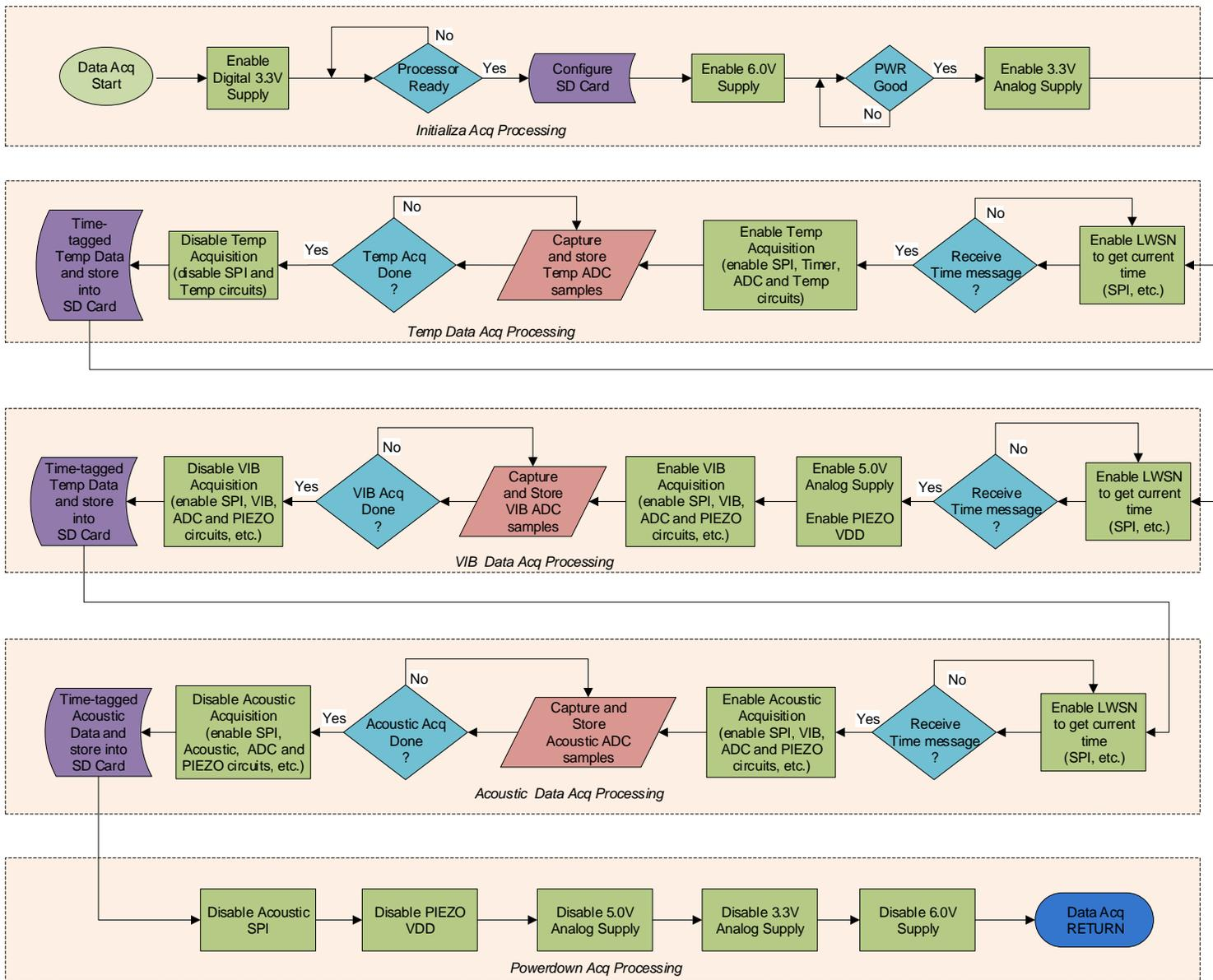
Figure 9. Data-acquisition process flow chart.
