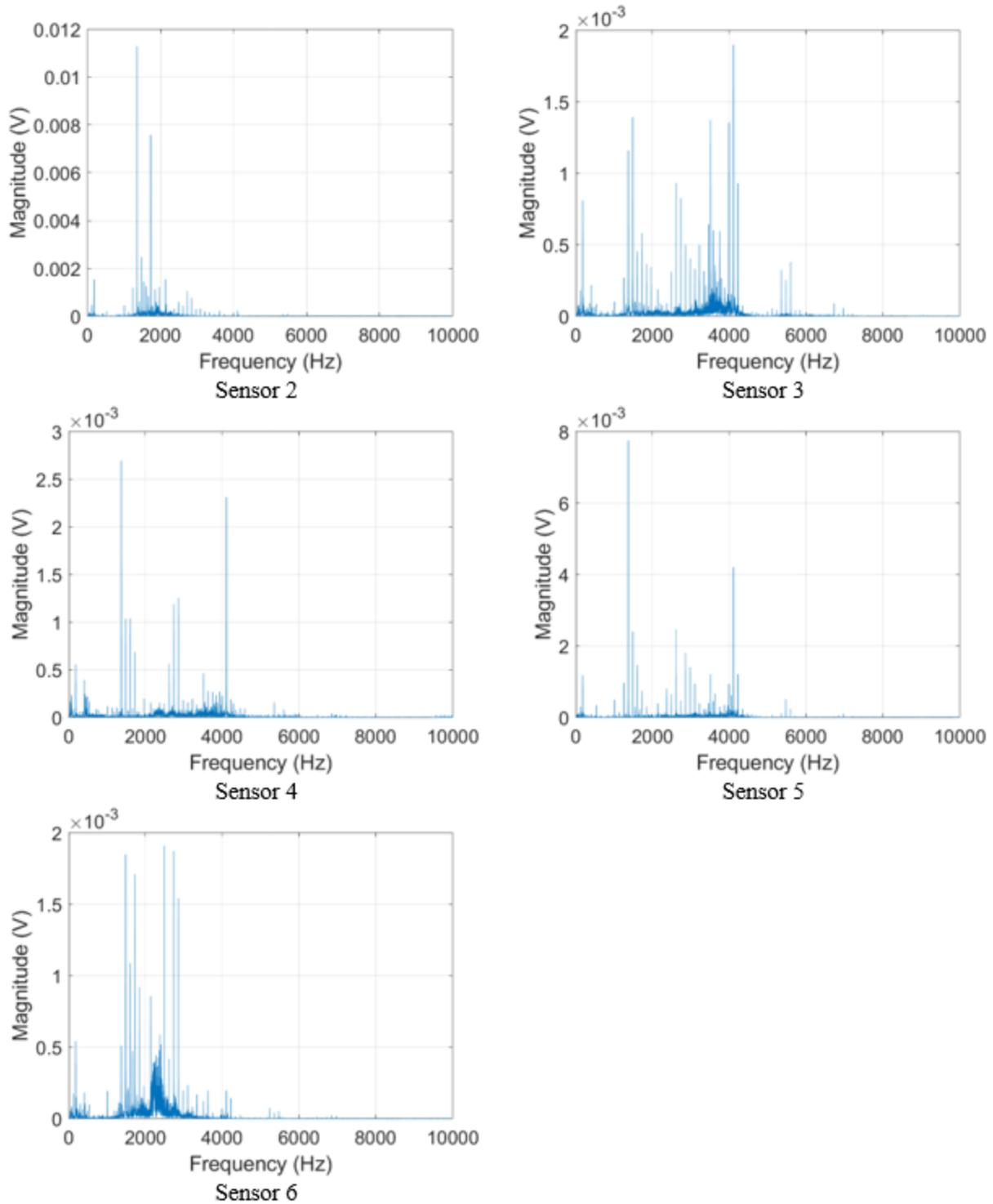
Figure 14. Vibration measured profiles in frequency domain (Sensors 2–6).
