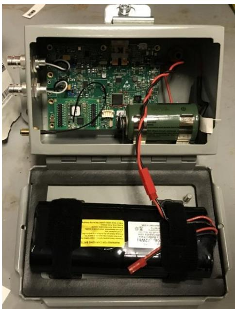
Figure 6. MSMU electronics board and battery (in black, mounted to the case).
