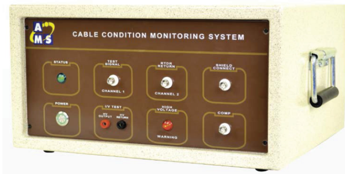
Figure 9.20. AMS CHAR system for monitoring cable condition. Courtesy of AMS Corporation.
