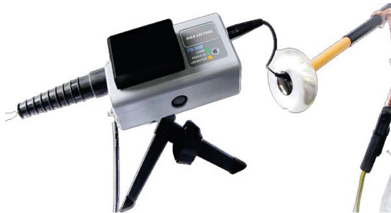
Figure 7.4. Tan Delta Model 34K. Photo courtesy of High Voltage Inc.
