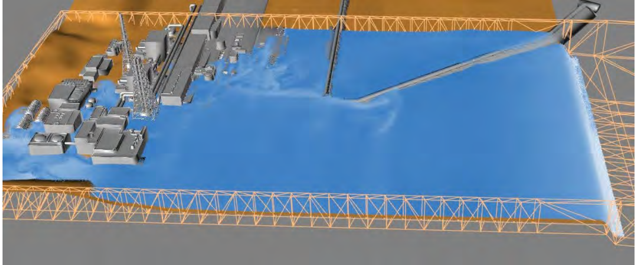
Figure 21: Half-facility tsunami simulation ~15 meters.
