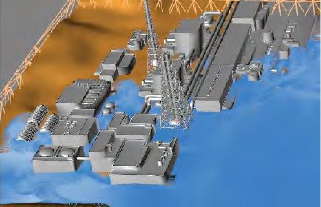
Figure 22: Close up view of the half-facility tsunami simulation ~15 meters.
