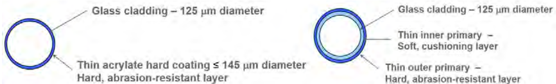
Figure 2. Single layer thin fiber coating geometry (left) and dual-layer thin fiber coating geometry (right).
