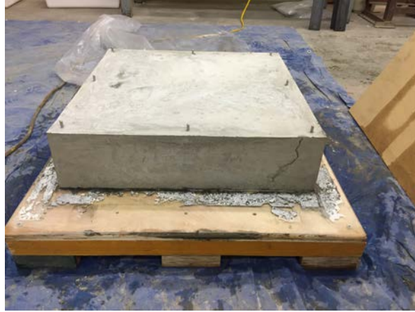
Figure 1. The plain concrete-slab specimen (dimensions 2 ft × 2 ft × 6 in.).
