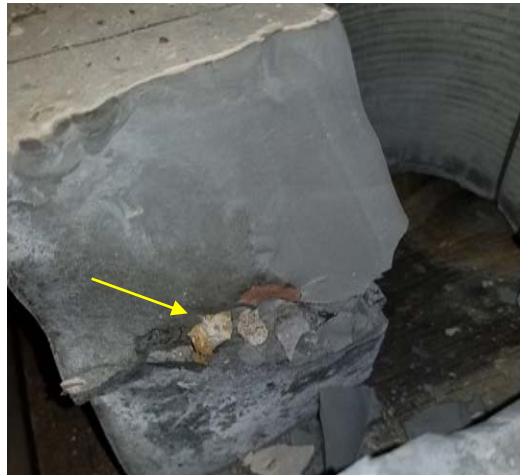
Figure 8: Shifting of aggregates and the presence of small hidden cracks in each quadrant of the plain concrete slab. (a) The shift of Maine aggregates in quadrant 1. (b) The amorphous silica in quadrant 2. (c) The spread of Ontario aggregates in quadrant 3. (d) The shift of New Mexico aggregates in quadrant 4.
