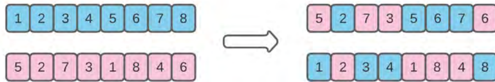
Figure 2-5. Schematic of the uniform crossover.
