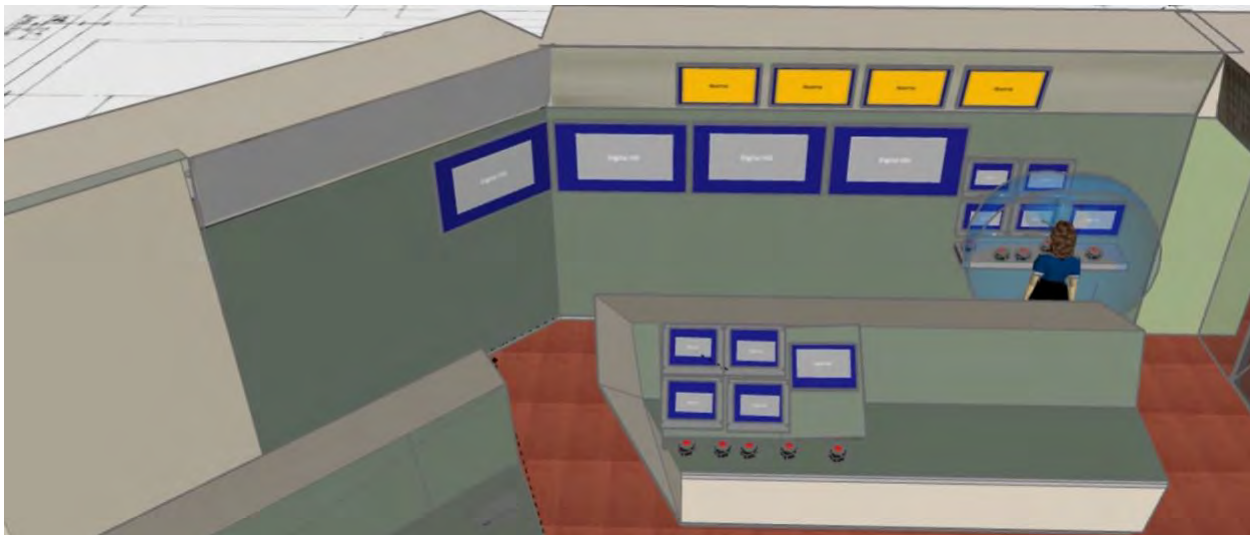
Figure 34. 3D model showing pre-task analysis modifications and 5th percentile female reach envelope.
