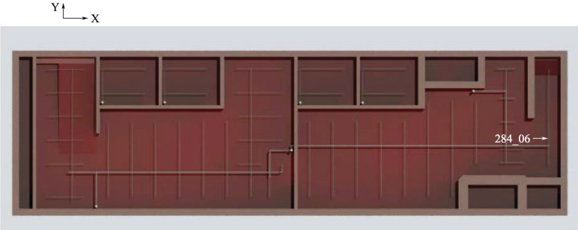
Figure 118 – Leakage Locations for the First Time History in Y Direction– PGA normalized to 0.9 g.
