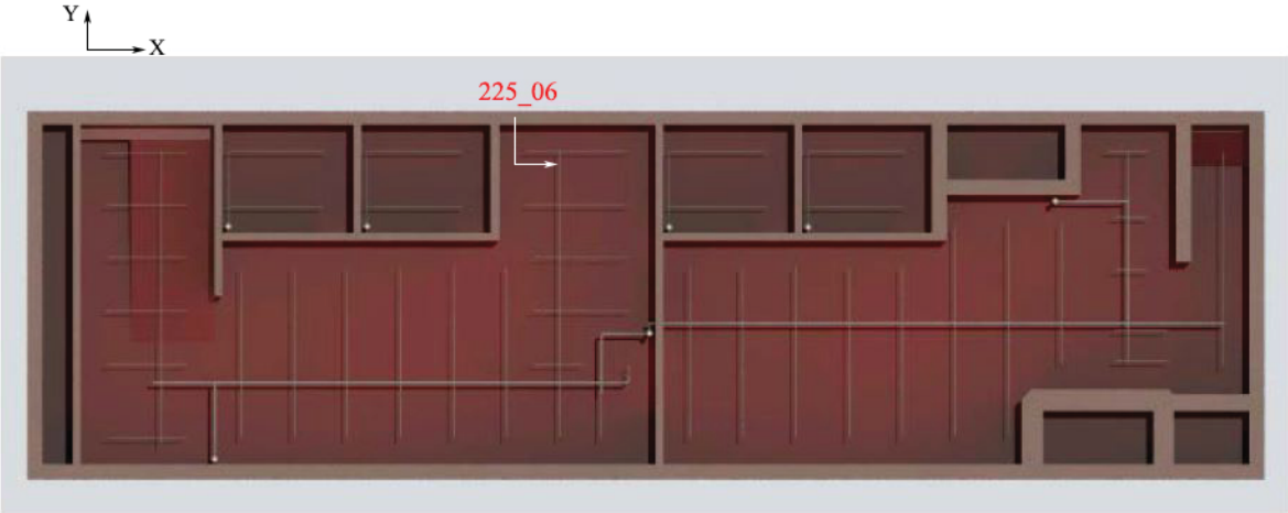
Figure 106 – Leakage Locations for the Third Time History in X Direction– PGA normalized to 0.6 g.
