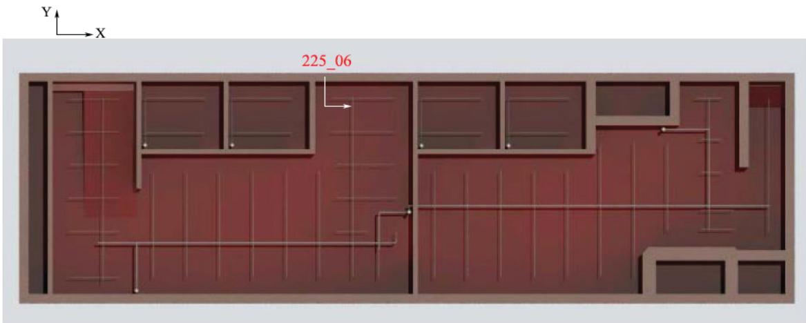
Figure 97 – Leakage Locations for the First Time History in X Direction– 0.297 g.
