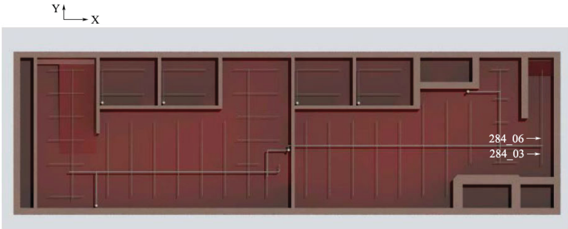
Figure 120 – Leakage Locations for the First Time History in Y Direction– PGA normalized to 1.5 g.
