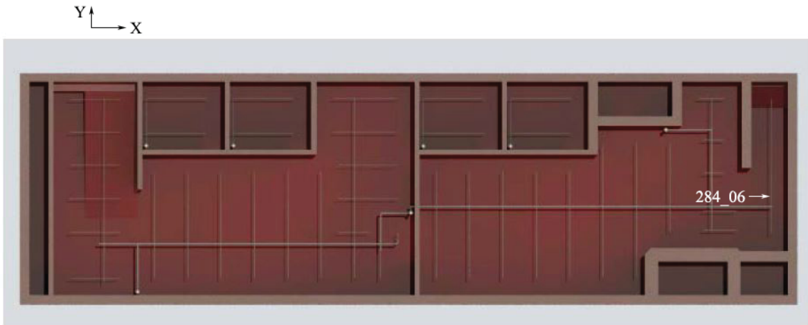
Figure 122 – Leakage Locations for the Second Time History in Y Direction– PGA normalized to 1.2 g.
