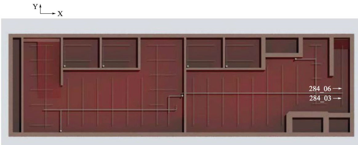
Figure 123 – Leakage Locations for the Second Time History in Y Direction– PGA normalized to 1.5 g.
