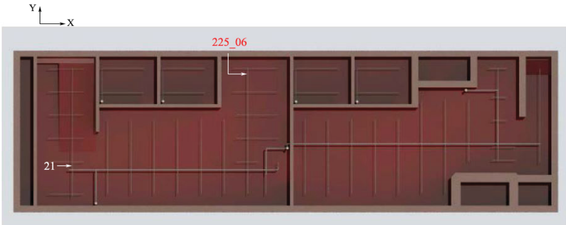
Figure 114 – Leakage Locations for the Fifth Time History in X Direction– PGA normalized to 0.6 g.
