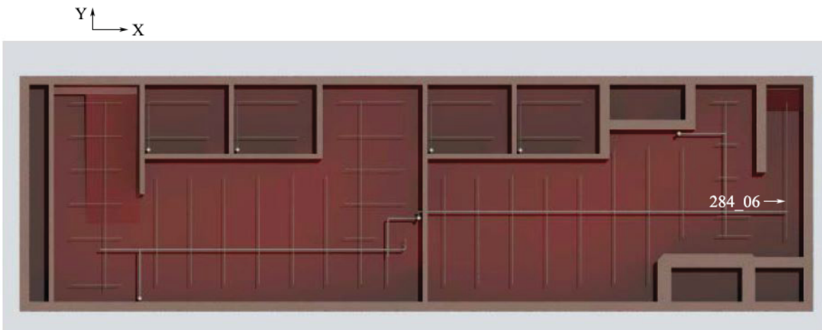
Figure 121 – Leakage Locations for the Second Time History in Y Direction– PGA normalized to 0.9 g.
