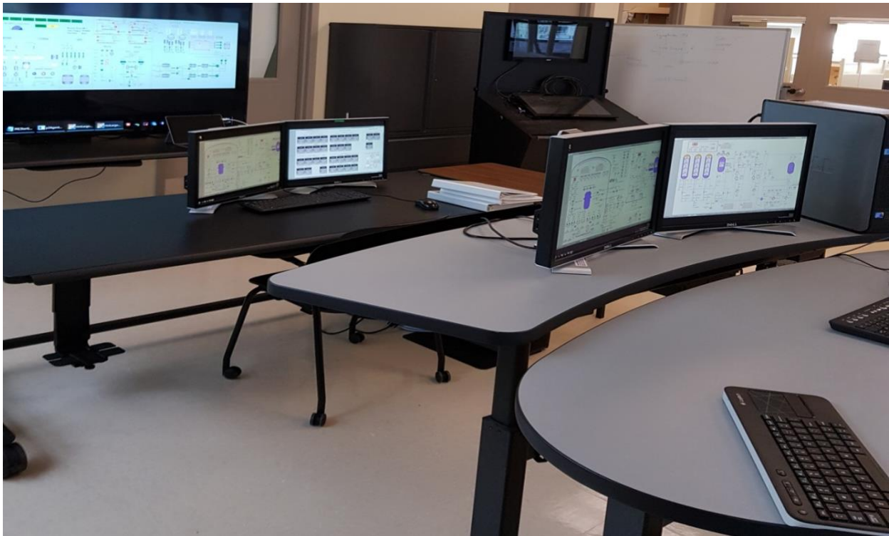
Figure 3. ACR two-man crew setup in HSSL.
