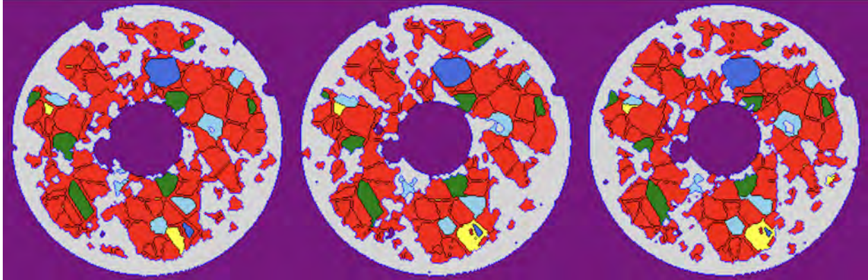
Figure 10. Three consecutive layers from the generated phase map: quartz (red), albite (orange), biotite (yellow), anorthite (sky blue), microcline (green), clinocllore (royal blue), IPI (black), ITZ (blue), hcp (light gray), and void (purple).
