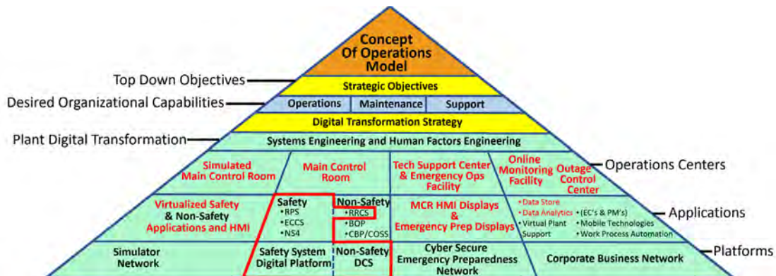
Figure 1. Advanced concept of operations model, with the Limerick Safety-Related I&C Pilot Scope outlined in red.
