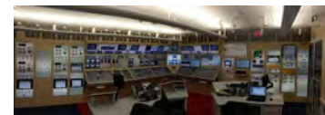
Leverage Glasstop Simulator for I&C Design, Procedure Development in Addition to Operator Training
