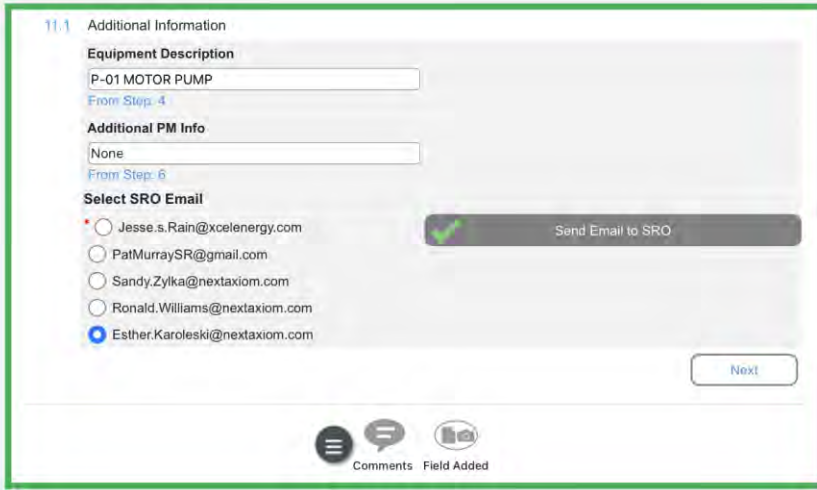
Figure B20. In the equipment scenario, the user confirmed the equipment description supplied by the backend system, and additional information provided by the user related to preventive maintenance. The user had the option to send a notification email to the SRO alerting them of the condition report by tapping the ‘Send Email to SRO’ button.
