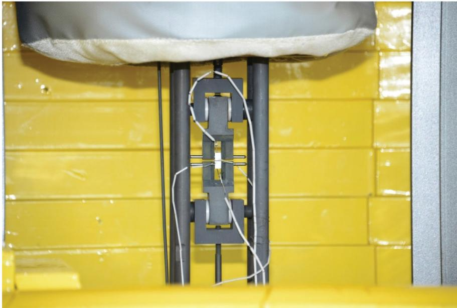
Figure A-4. Specimen loaded in the autoclave and ready to be tested.
