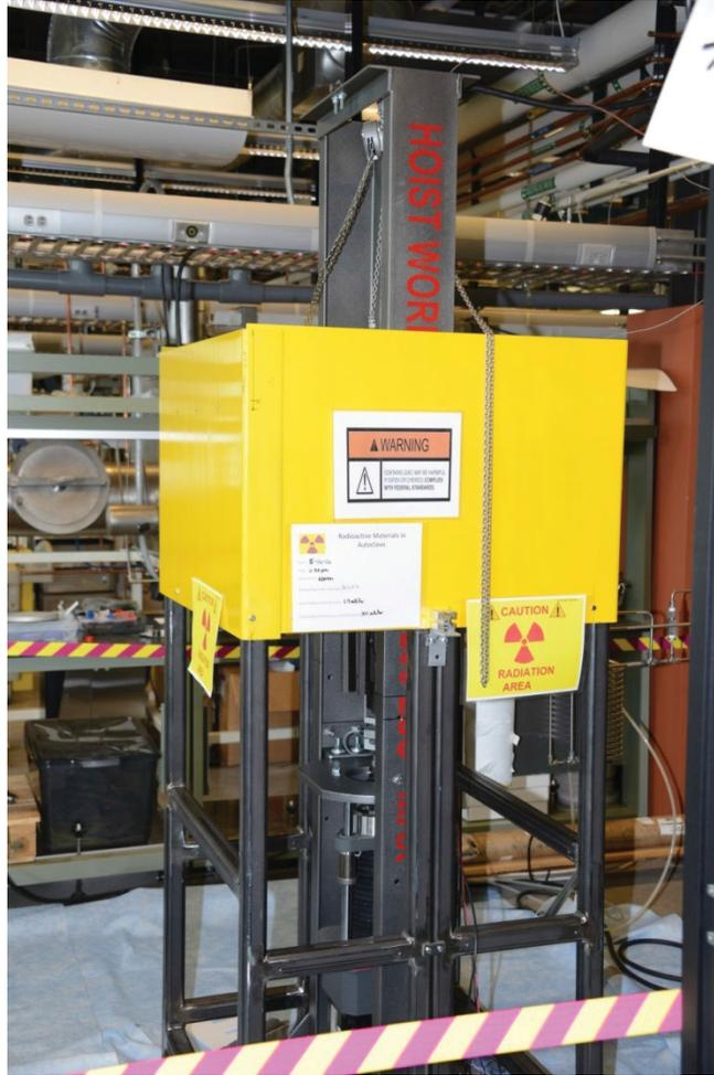
Figure A-5. IASCC testing jig with shield closed.
