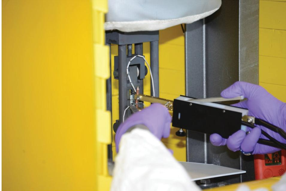
Figure A-3. The direct current potential drop leads being connected to the samples leads.
