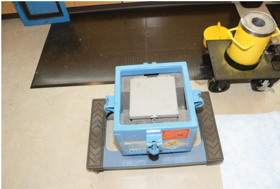
Figure A-7. The shipping container (in blue) contains the specimens. Those specimens will be transferred to the yellow lead pig for storage and transport within the testing facility.
