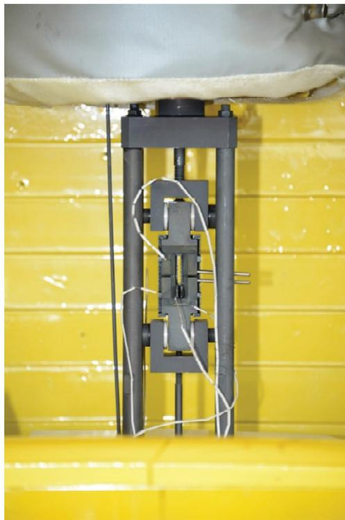
Figure A-2. Clevises and guiding jig prepared before loading the specimen.
