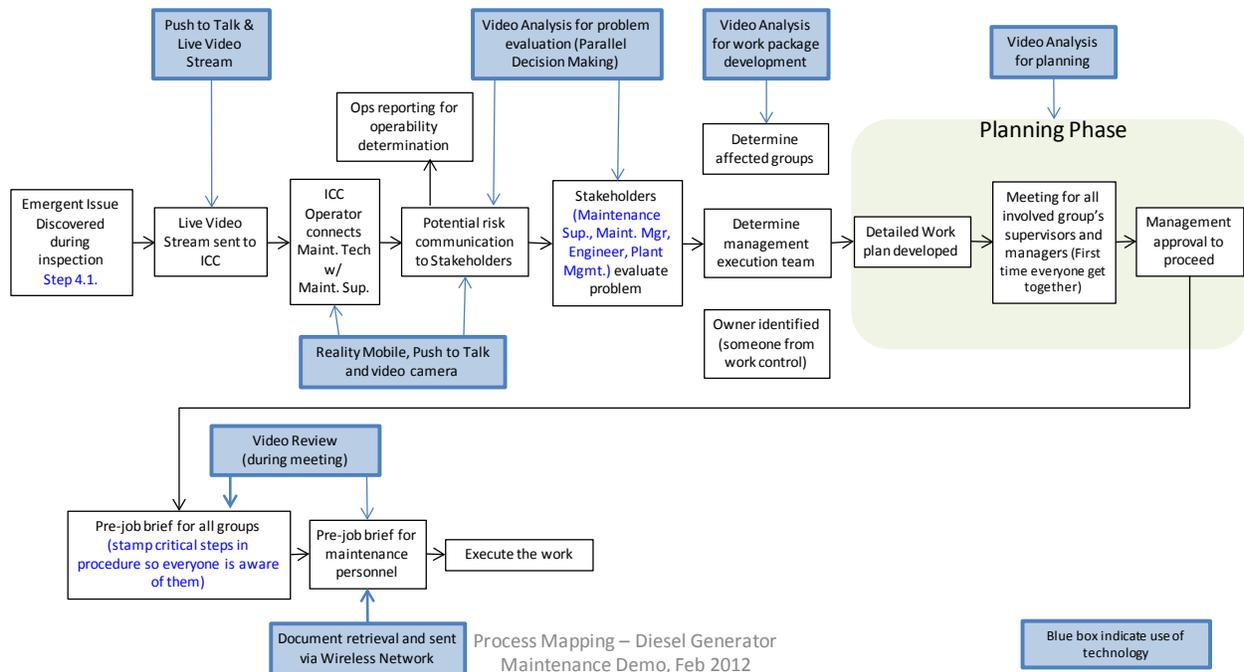
**Figure 4. Diesel generator maintenance demonstration process map.**
