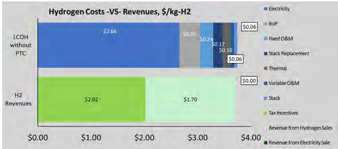
Figure 13. The input parameters and financial performance for Case 3 with 500 MW-dc of HTSE design capacity, 20 years of plant life, 12.10% of WACC, $3/kg PTC, NG-correlated hydrogen market price, and regulated NG-correlated electricity price.
