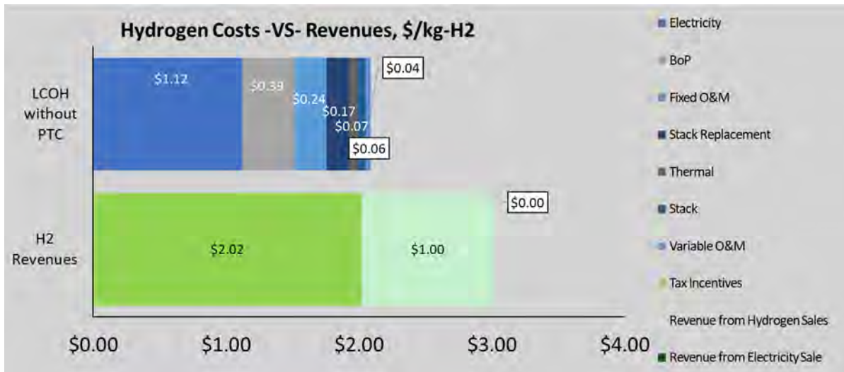
Figure 8. LCOH and revenue breakdown for Case 2 with 500 MW-dc of HTSE design capacity, 20 years of plant life, 12.10% of WACC, $3/kg PTC, hydrogen market price of $1.10/kg-H 2 , and $30/MWh of regulated electricity price.
